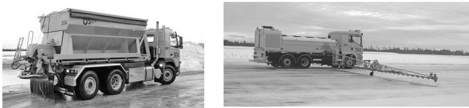
Photo 5. a) Spreader, b) sprayer
