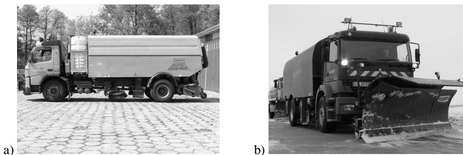
Photo 6. a) airport vacuum cleaning machine, a side view, b) airport vacuum cleaning machine with a snowplough attached
