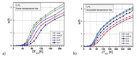
Fig. 1. Maximal deflection of the plate vs. dynamic thermal loading for a) linear temperature rise and b) sinusoidal temperature rise
