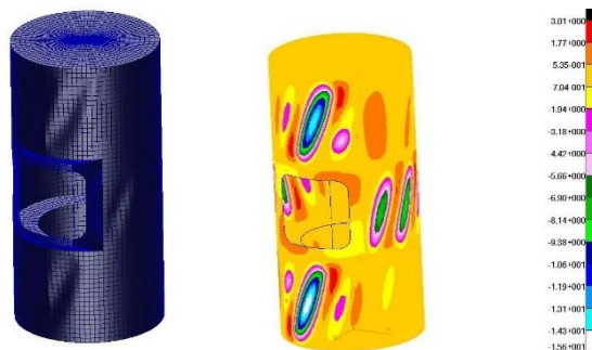
Fig. 3. The pattern of post-critical displacements (left) and resultant displacement distribution (in mm) (right)
