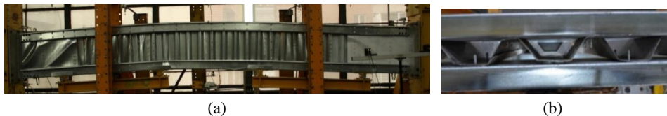
Fig. 1. (a) Deformed shape of CWB-5 beam at failure; (b) the distortion of the web corrugation
