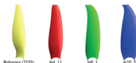
Figure 1. Investigated propeller blades: reference (TUD) and optimized (Ł-ILOT)
