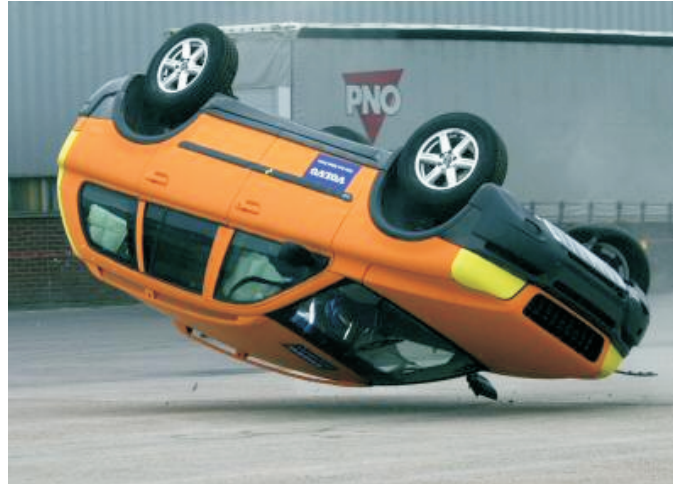
Figure 9 Rollover crash test of Volvo XC90 [7]
