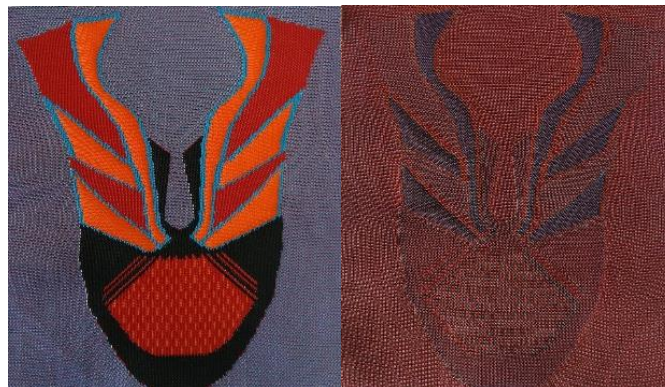
Figure 1. View of the right and left side of the upper part of the footwear produced on a large diameter cylindrical crochet machine (option 1).
