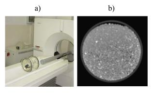
Fig.3. X-ray tomography: a) specimen prepared for test, b) tomogram (vertical cross-section)
