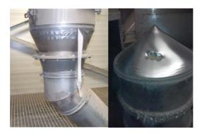
Fig. 2. Example of mechanical damage to the magnetic conical separator *Source: own elaboration.*
