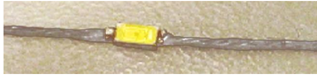
Figure 1. SMD LED embedded Steeliness steel E-yarn.
