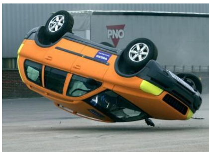
Fig. 9. Rollover crash test of Volvo XC90 [7]
