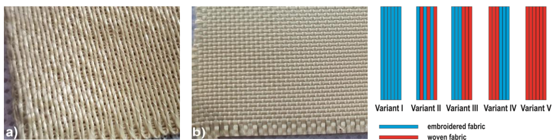
Figure 1. The method of making ballistic packages: a) embroidered structure, b) Twaron CT 709 fabric, c) variants of ballistic packages.
