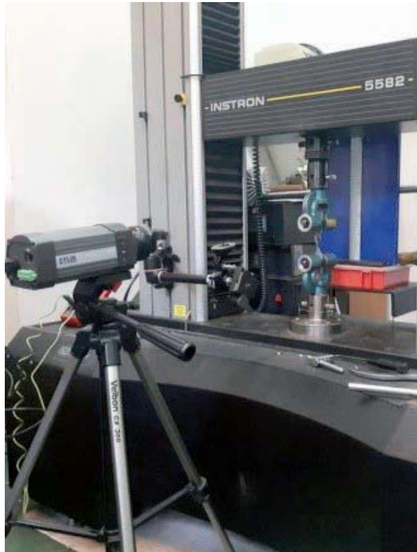
Fig. 2. Tensile strength test of polyurea - test bench.
