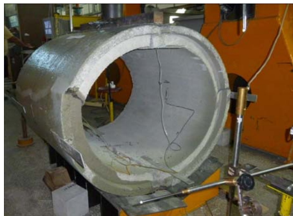
Fig. 10. Concrete ring after failure: type II.
