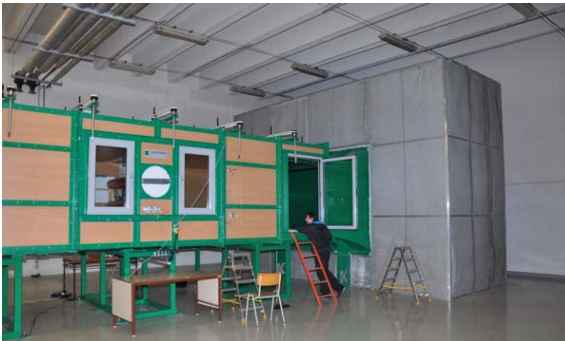
Fig. 3. Air filter and laminar flow section of the wind tunnel.
