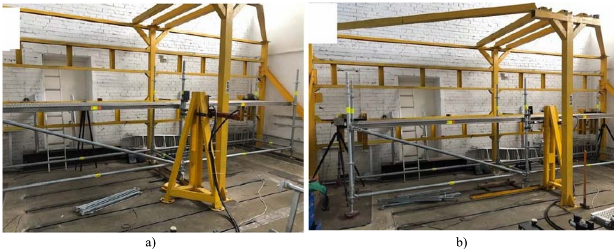
Fig. 6. Test stands for (Misztela (2020)): a) platforms with a perpendicular load; b) platforms with a parallel load.
