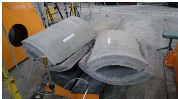
Fig. 9. Concrete ring after failure: type I.
