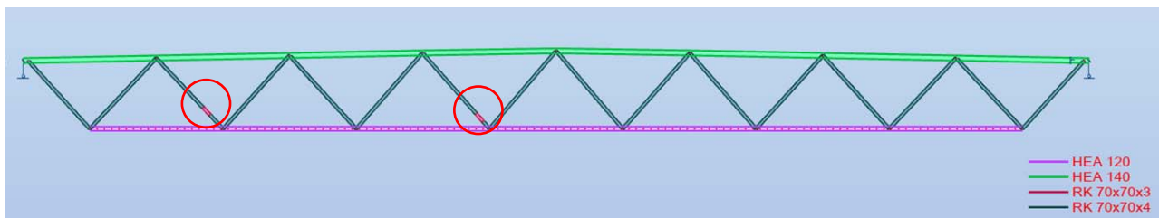
Fig. 11. The places of introduction of the weakening cross-sections in the relation to the entire girder.
