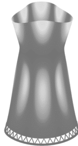
Fig. 7 – First modal shape of natural vibration
