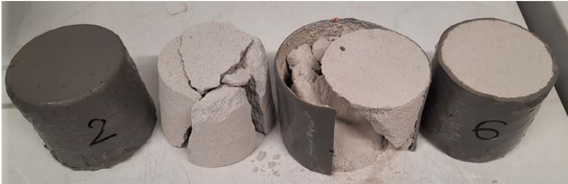
Fig. 8. Cellular concrete samples after the failure.
