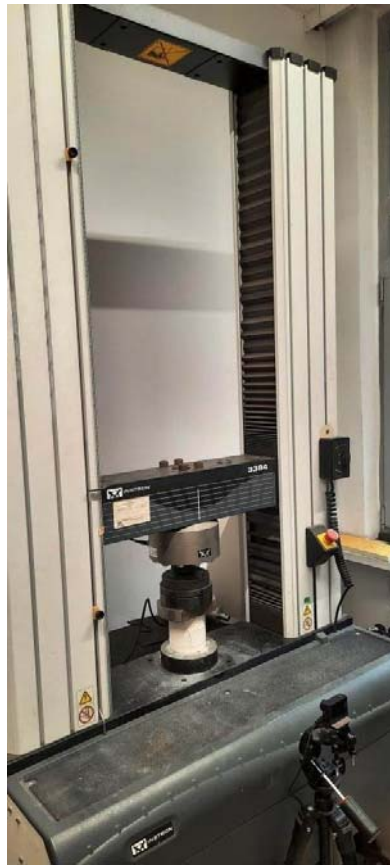
Fig. 6. Compressive strength test of cellular concrete - the test bench.
