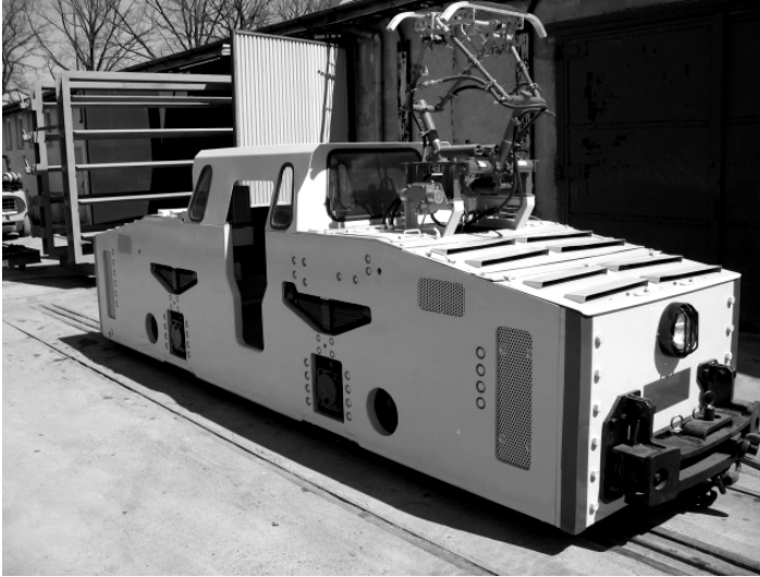
Fig. 3. Mining locomotive Ld-31 EM with PMSM produced by Komel [7] The company exists since 1948 as an independent testing center and builds its own prototypes, and is ready to apply traction drives, Fig 3 and 4
