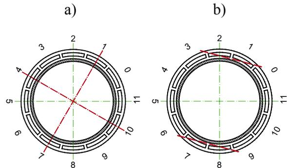
Fig.4. 12-electrode sensors used during experiments with ECT, examples of the cross-section profiles a) between electrodes 1-7 and 4-10; next close to the wall profiles b) between electrodes 1-2 and 7-8
