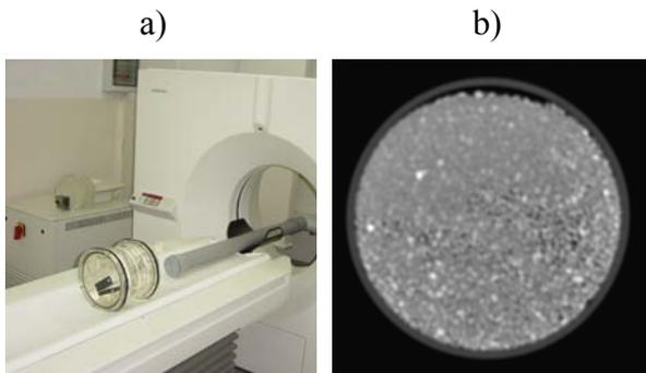
Fig.3. X-ray tomography: a) specimen prepared for test, b) tomogram (vertical cross-section)
