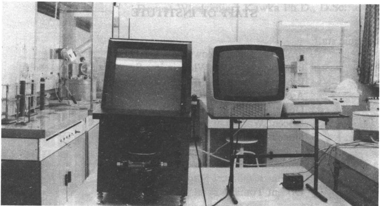
Apparatus for fibre length measurement developed in the Institute
