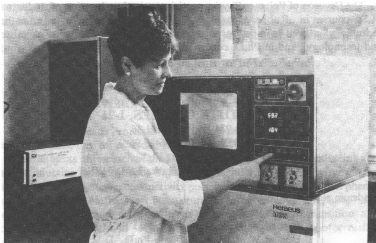
Xenotest - apparatus for testing of light-fastness of dyeing
