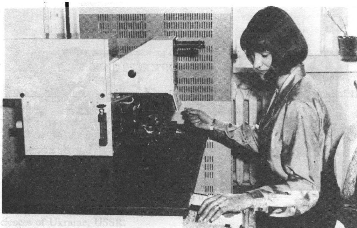
Impulse laser for spot- welding
