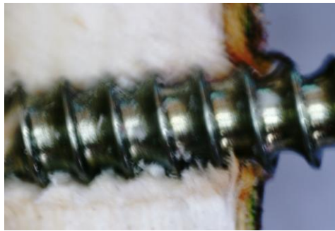
Figure 2. Image of the contact geometry at the boundary of the living structure and the artificial material: a steel screw mounted within a tree – magnification of 200x
