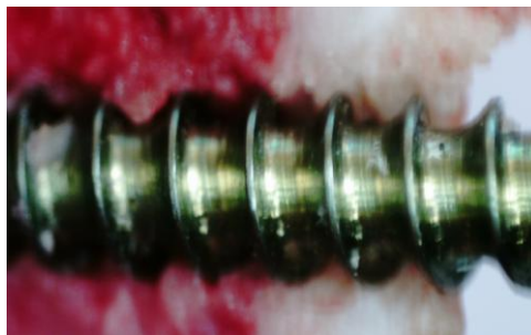
Figure 1. Image of the contact geometry at the boundary of a living structure and an artificial material: a steel rod mounted within a bone – magnification of 200x
