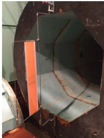
Figure 4. Double aerodynamic pendulum in wind tunnel.
