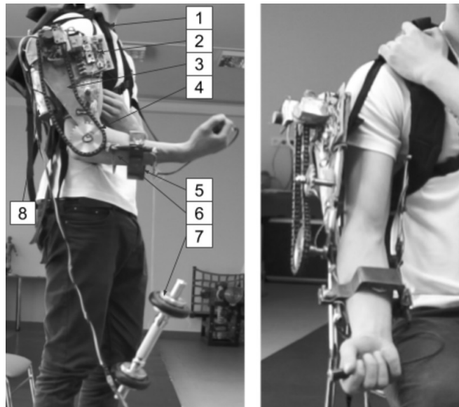
Figure 4. The arm exoskeleton prototype: 1 - straps, 2 - controller, 3 - arm part of the exoskeleton, 4 - chain transmission, 5 - braces with pressure sensors, 6 - forearm part of the exoskeleton, 7 – weight, 8 - motor with reducer.
