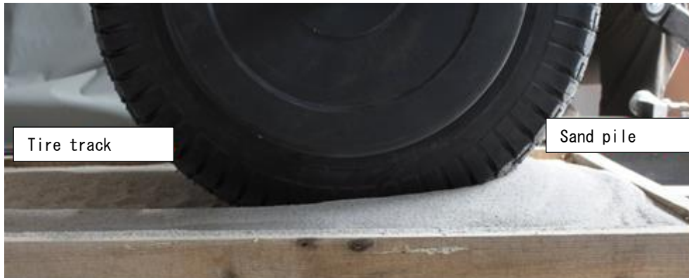
Figure 10. The wheel on the experimental stand, after test with \alpha_w = 0^\circ .
