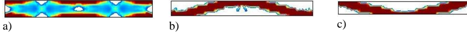
Figure 2. Optimal beam topologies: a) T_{opt} = 20^0 C , b) T_{opt} = 50^0 C , c) T_{opt} = -30^0 C
