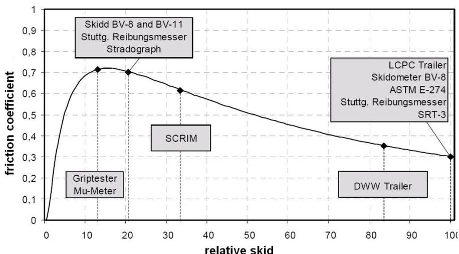
Fig. 2. Diversification of the methods of measuring the friction coefficient with exemplary measurements<sup>18</sup>
