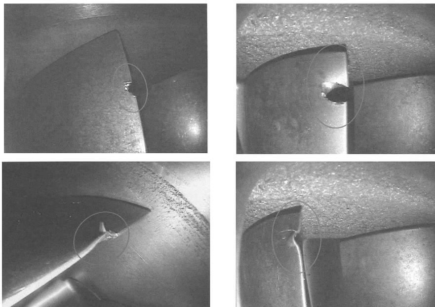
Photo 1. Damage to the blades of a MIG-29 compressor after sucking contamination
