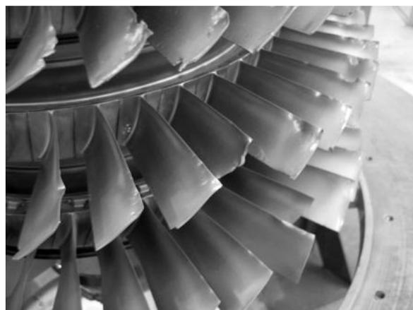
Photo 2. Damage to the blades of a Boeing 757-200 compressor
