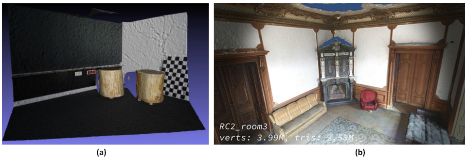
Fig. 7. A sample reconstruction of a flat surface illuminated by a graphical pattern from an LCD projector (a), a sample reconstructed scene imported into Unity 3D environment (b)
