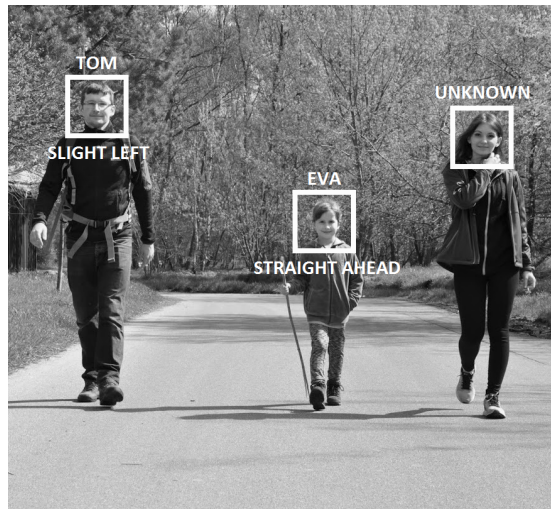
Fig. 3. The Face Navigator application view – analysing from the left: person 1 – TOM: SLIGHT LEFT; person 2 – EVA: STRAIGHT AHEAD; person 3 – UNKNOWN
