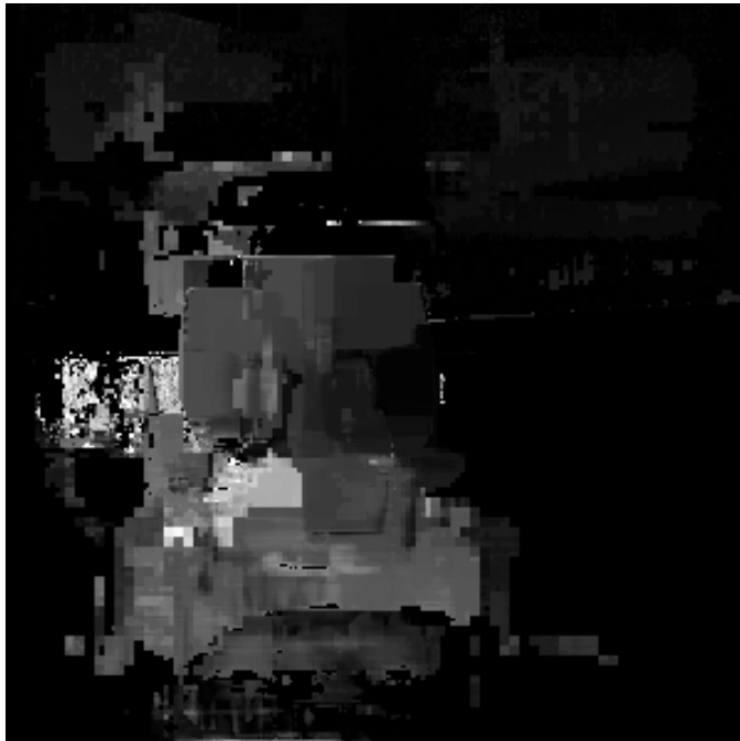
Fig. 3. The magnitude of optical flow vectors obtained from consecutive frames as presented in Fig. 1. Black represents the magnitude of 0, while white represents a magnitude of 128 pixels or above. Note, that the magnitude is presented in the frame of the preceding image (left one in Fig. 1)
