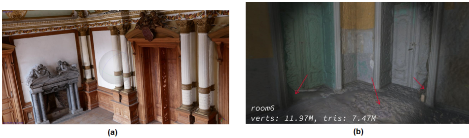
Fig. 3. Sample results from Agisoft Photoscan: a textured fragment of a room (a), geometry distortions on flat surfaces in a corridor (b)
