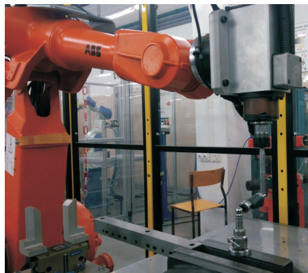
Figure 3 Robot IRB 2400 with telescoping ball bar
