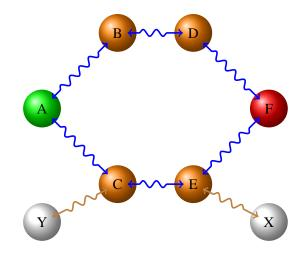
Figure 4. A topology similar to depicted on Figure 3, where nodes C and E are slightly moved to prefer path ACEF. The topology is augmented by nodes X and Y, where node X transmits data to node Y between 10th and 30th second of simulation. Background traffic is exactly the same as in previous example.
