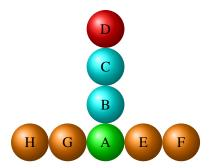
Figure 1. Node A broadcasts message with DA=D. Finally nodes B and C have to relay message, while the E, F, G and H ones should drop it. Nodes B, E and G are in range of A; none path is known by any node at any time.
