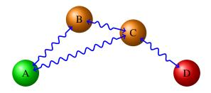
Figure 2. Node A broadcasts message with DA=D. Budget on path ABCD is approximately the same as on path ACD, which should be the preferred one.
