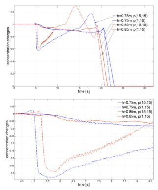
Fig. 8. The concentration changes during the silo discharging for initially dense packing with the smooth silo wall, dense sand, height of sensor position (h=0.75m and 0.85m) and analysing point selection (centre or close to the wall) like on legends.
