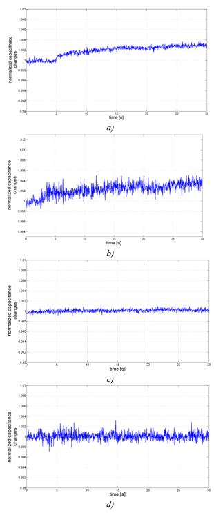
Fig. 3. Normalized capacitance changes (the opposite electrodes) in funnel area for sensor located at 1m and 0.3m above the outlet with controlled discharging - velocity v=0.1mm/s: a) loose sand, measured on 1.0 m; b) loose sand, measured on 0.3 m; c) dense sand, measured on 1.0 m; d) dense sand, measured on 0.3 m.
