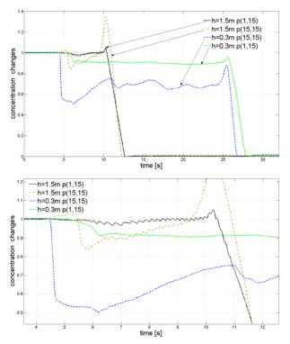
Fig. 6. Concentration changes during the silo discharging for initially dense packing sand with the smooth silo wall, height of sensor position and analysed point selection like on legends.
