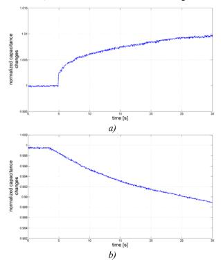
Fig. 4. Normalized capacitance changes (the adjacent electrodes) in stagnant zone, for sensor located at 1m above the outlet with controlled discharging - velocity v=0.1mm/s: a) loose sand; b) dense sand
