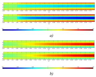
Fig. 5. Topograms - the sequence of vertical cross of tomography images in time, controlled velocity of discharging 0.1 mm/s, measurement on h=1.0m: a) smooth wall, loose sand; b) smooth wall, dense sand
