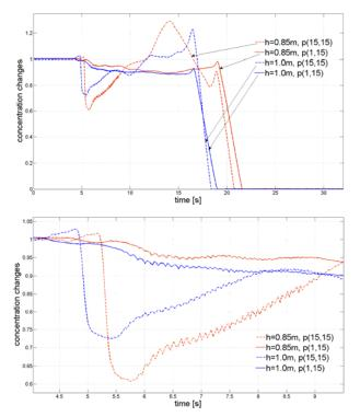
Fig. 9. The concentration changes during the silo discharging for initially dense packing with the smooth silo wall, dense sand, height of sensor position (h=0.85m and 1.0m) and analysing point selection (centre or close to the wall) like on legends.
