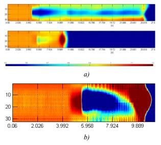
Fig. 7. Topograms - concentration changes in the whole length of sensor cross-section, b) h=0.3m and h=1.5m, b) magnification emphasizes the oscillations for h=1.5m in fig. 6
