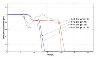
Fig. 10. The concentration changes during the silo discharging for initially dense packing with the rough silo wall, dense sand, height of sensor position (h=0.3m and 1.5m) and analysing point selection (centre or close to the wall) like on legends.
