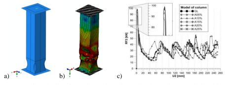
Fig. 1. Subject of analysis: a) - theoretical model (A15%), b) - numerical model - failure pattern, c) - comparative load-shortening diagram
