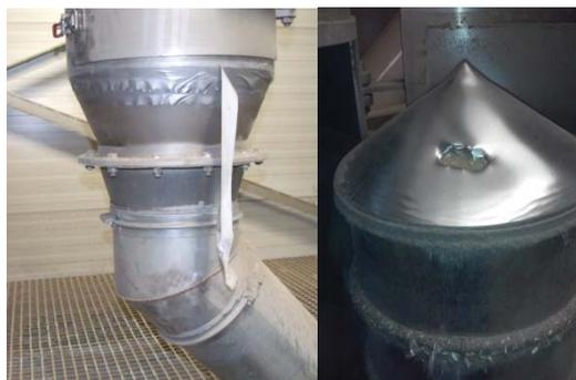
**Fig. 2.** Example of mechanical damage to the magnetic conical separator
