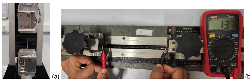
Figure 2. J. H. - Universal strength tester with “120 N loading cell” (a), conductivity tested by UNI-T UT33B digital multimeter on a J. H. Tensile Testing Equipment with increments of “5% elongation” (b).
