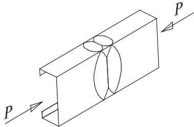
Fig. 9.6. Plastic mechanism of failure for lipped channel section in compression [9.4]
