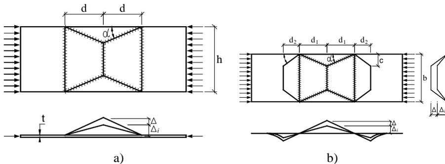
Fig. 9.4. Plastic mechanisms in thin plates under compression: a) pitched-roof, b) roof
