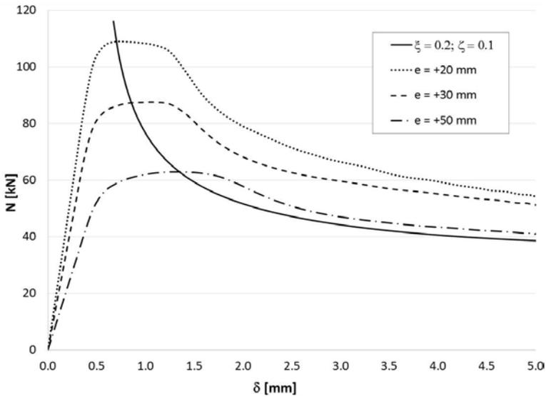
Fig. 9.13. Load-shortening diagrams for large positive eccentricities
