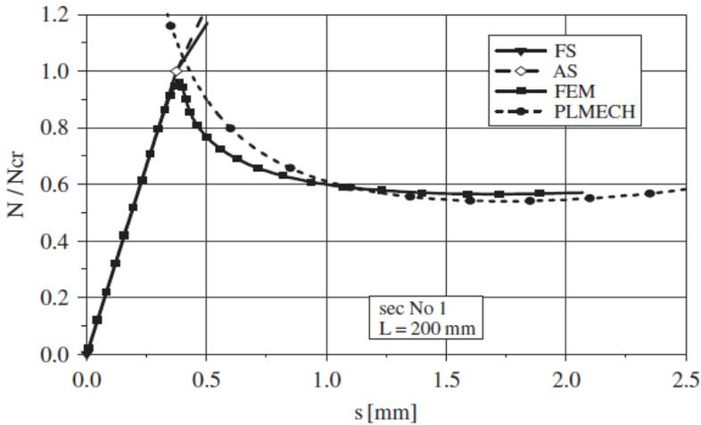
Fig. 9.9. Structural behaviour of the top hat section:  $a = 50$ ,  $b = 33.5$ ,  $w = 12.5$ ,  $t = 1$  [mm],  $\sigma_Y = 480$  Mpa [9.31]
