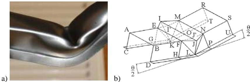
Fig. 9.8. Plastic mechanism of failure for a top hat sections [9.26]: a) real mechanism of failure (quasi-static test), b) theoretical model
