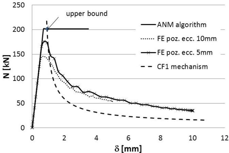
Fig. 9.11. Load-shortening diagrams for small positive eccentricities
