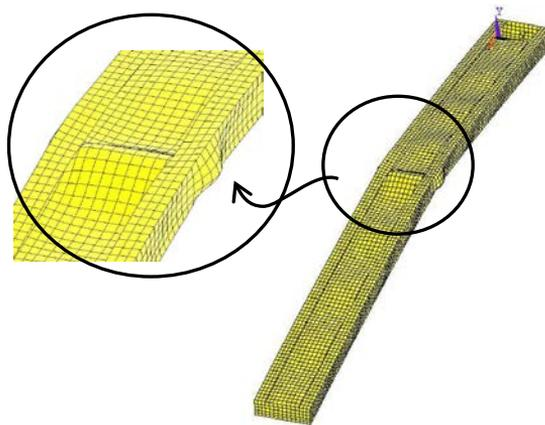
Fig. 9.3. FEM simulation of plastic-elastic interaction between the local plastic mechanism and global buckling for a lipped channel section in compression [9.3, 9.4]
