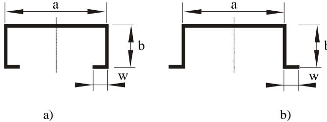
Fig. 9.5. Members with edge stiffeners: a) lipped channel section, b) top hat section
