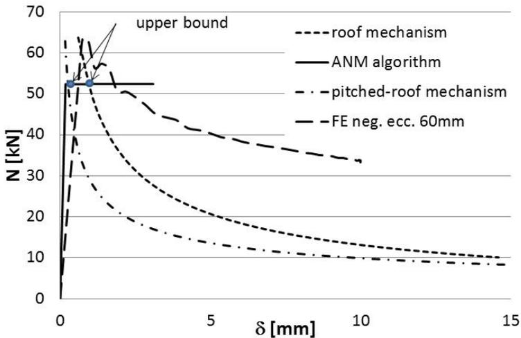
Fig. 9.14. Load-shortening diagrams for large negative eccentricities
