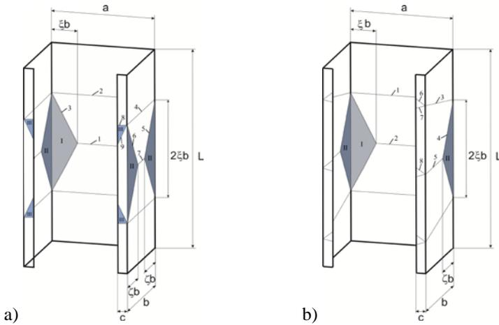
Fig. 9.7. Theoretical models of: a) “triple-roof” mechanisms, b) CF-quasi-mechanism
