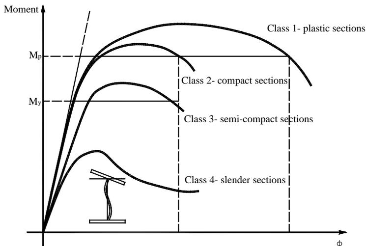
Fig. 9.1. Cross-section behaviour classes
