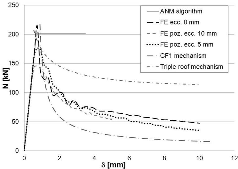
Fig. 9.12. Load-shortening diagrams for small positive eccentricities - comparison for two mechanisms
