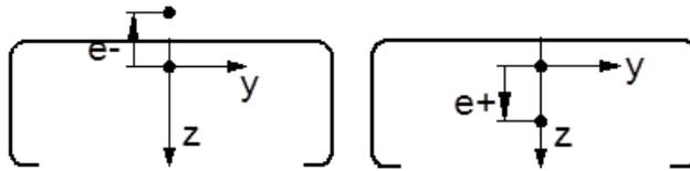
Fig. 9.10. Lipped channel sections with negative and positive eccentricities
