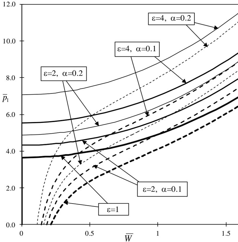
Fig. 3. Relations between uniaxial compression and maximum macrodeflection of initially flat (solid lines) and deflected due to transversal load (dashed lines) square plates
