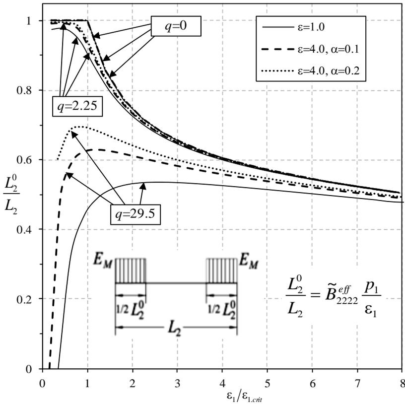
Fig. 4. Effect of transversal load on effective width of a square plate loaded by edge compression
