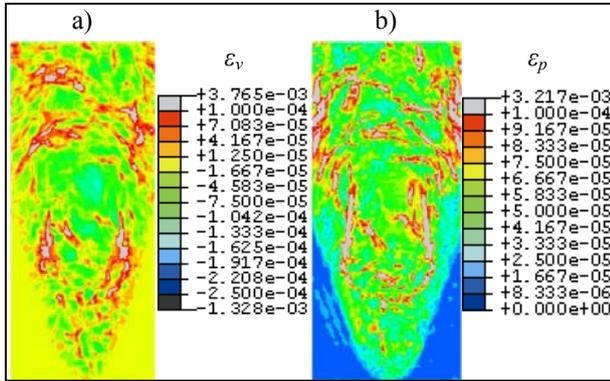
Fig.3: Evolution of the volume strain  $\varepsilon_v$  (a) and deviatoric strain  $\varepsilon_p$  (b) in a mass flow silo after 7 s of flow for the rough wall silo
