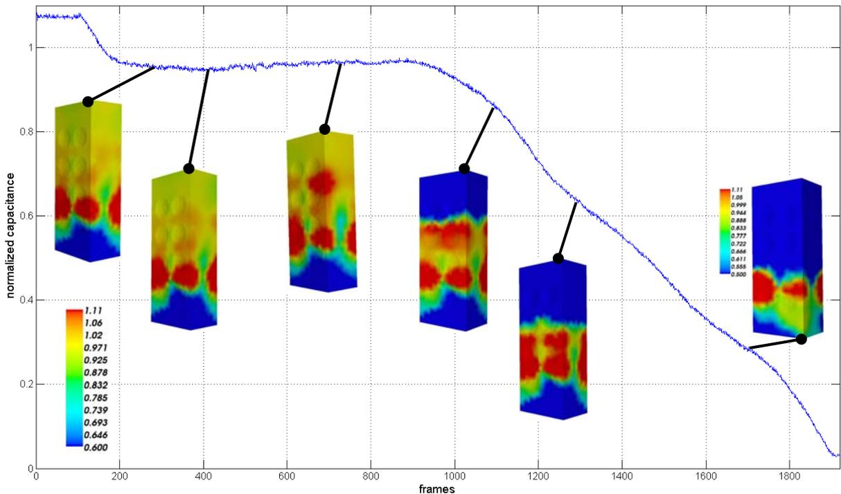
Fig. 7. Characteristic plot of the silo discharging process illustrated additionally with 3D images corresponding to several phases (distinct points indicated on the plot) of the process. The case for sandpaper with grit size 16 (extra course) stick to the silo wall.
