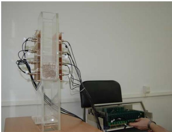
Fig.4 Laboratory silo model and ECT system photo.
