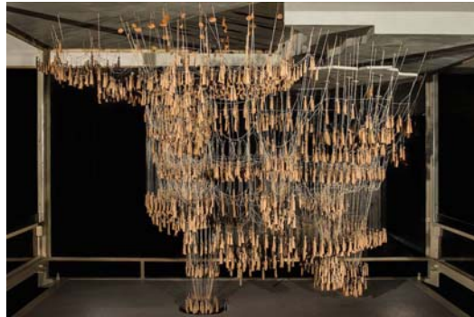
Fig. 1. Multidirectional model of the Colònia Güell church by Antoni Gaudi, 1898-1908.
