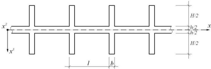
Fig. 2. A fragment of a cross-section of the stiffened plate structure
