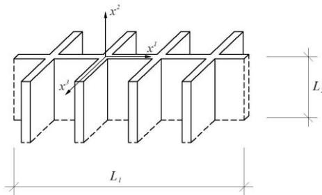
Fig. 1. A fragment of a plate structure with periodic system of stiffeners
