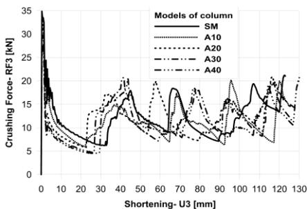
Fig. 2. Comparative load-shortening diagram
