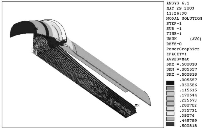
Fig. 3. Total strains of the heat exchanger [mm]
