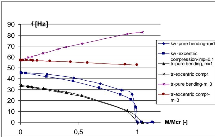
Fig.9. Frequencies of forced vibrations vs. moment ratio:  $M/M_{cr}$
