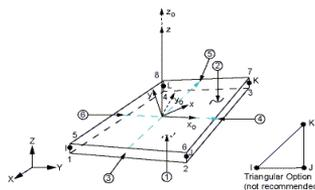
Fig. 1. SHELL99 element geometry [1]
