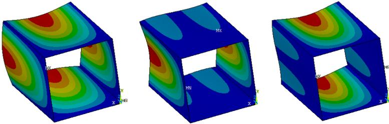
Fig.7. Modes of natural vibrations (half model) for rectangular beam
