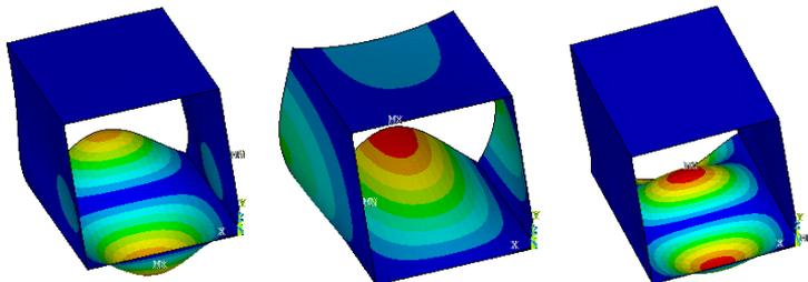
Fig.4. Buckling modes (half model) - for eccentric compression case: 1-3 modes (numbering from left to right)
