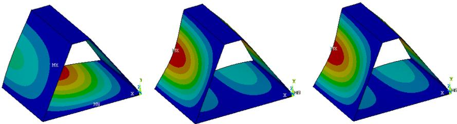
Fig.8. Modes of natural vibrations (half model) for trapezoidal beam
