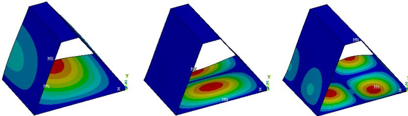
Fig.6. Buckling modes (half model) - for eccentric compression case: modes 1-3 (numbering from left to right)
