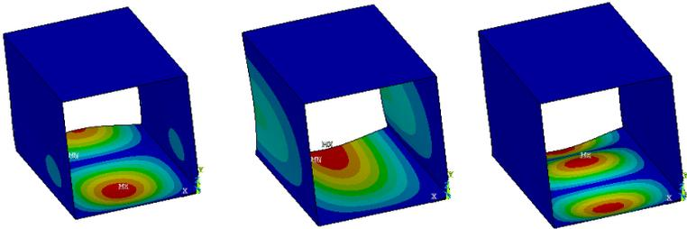
Fig. 3. Buckling modes (half model) - for pure bending case: modes 1-3 (numbering from left to right)
