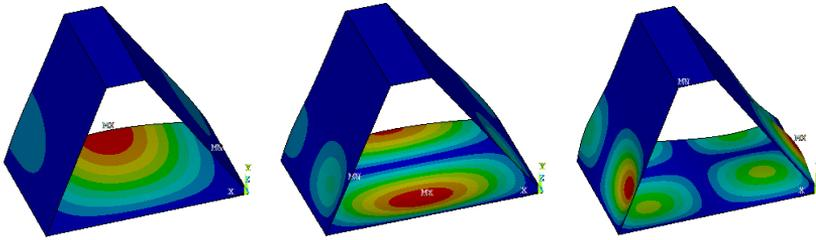
Fig.5. Buckling modes (half model) - for pure bending case: modes 1-3 (numbering from left to right)
