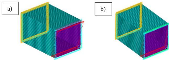
Fig. 2.1. Numerical model and boundary conditions (half model): a) pure bending, b) eccentric compression
