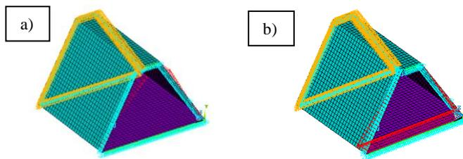
Fig. 2.2. Numerical model and boundary conditions (half model) for two cases of load: a) pure bending, b) eccentric compression
