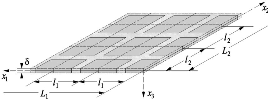
Fig. 1. Fragment of a thin periodic plate
