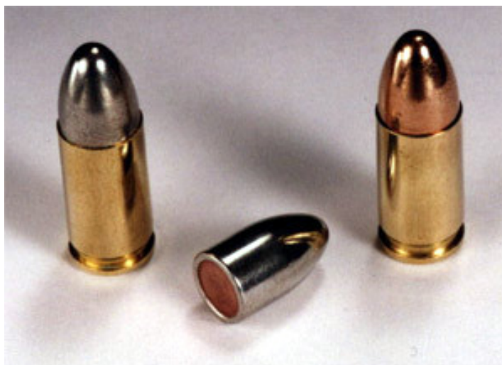
Rys. 5. Pocisk PARABELLUM 9 × 19 mm FMJ [11]
