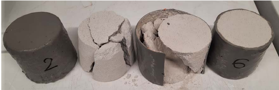
Fig. 8. Cellular concrete samples after the failure.
