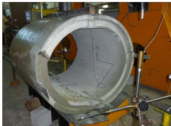
Fig. 10. Concrete ring after failure: type II.
