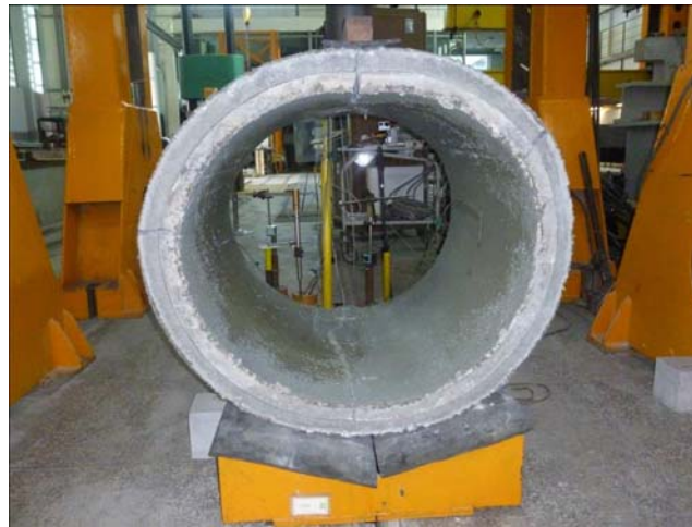
Fig. 11. Concrete ring after failure: type III.
