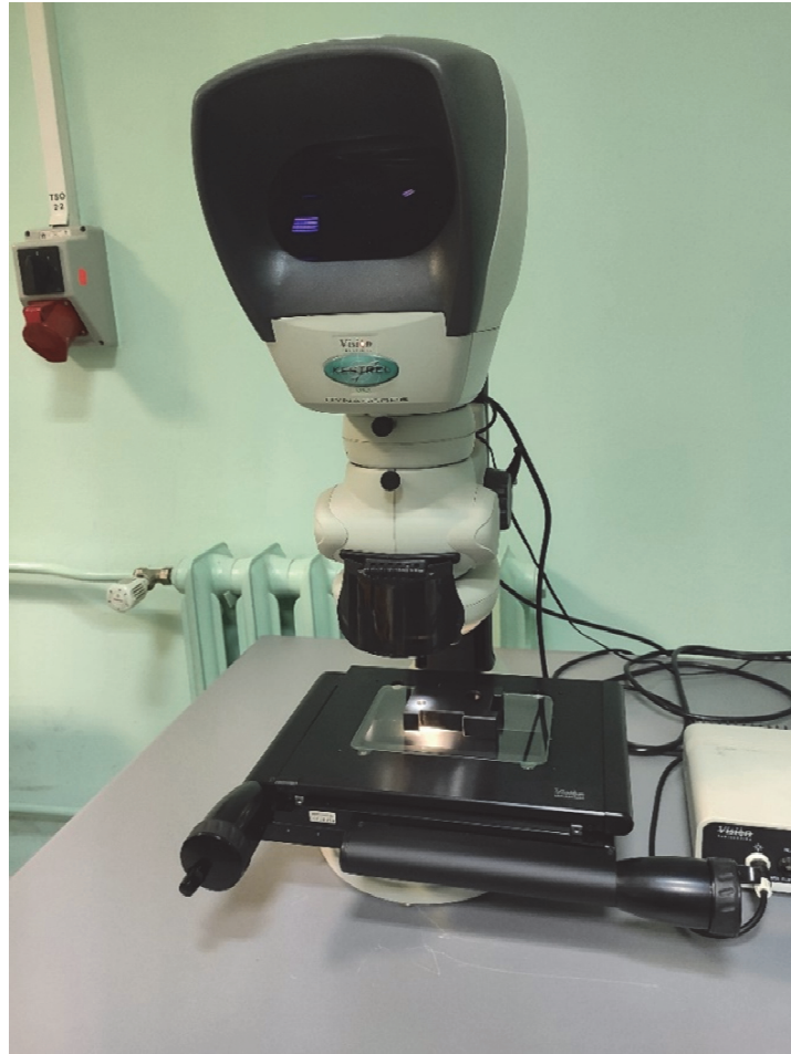
Figure 8.14. Electronic version of Tool work microscope QC300 from Vision Engineering
