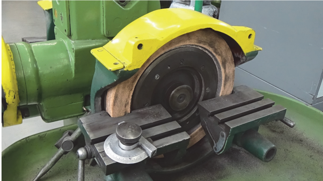
Figure 10.5. Single-point turning tool sharpener (double scale sharpening device)
