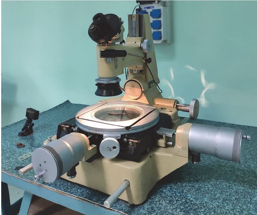
Figure 8.13. Toolroom microscope MWD – laboratory equipment
