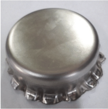
Figure 11.3. Deep drawing operation -wrinkling example [3]
