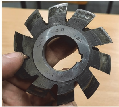
The effect of improper grinding of the rake surface on the shape errors of the teeth cut:
