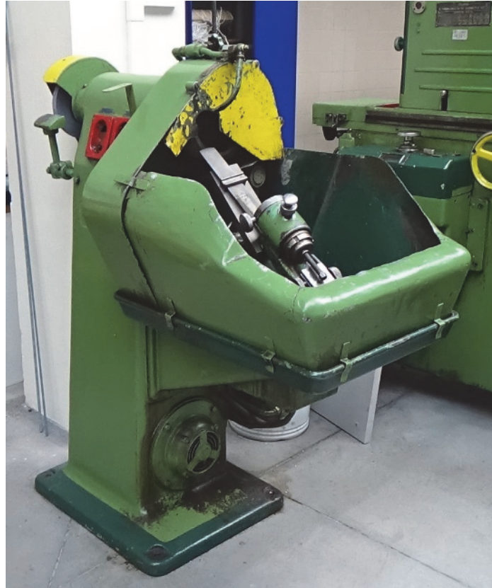
Figure 10.13. Twist drill sharpener from Malcus corporation (Sweden)
