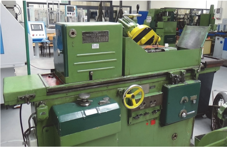
Figure 10.21. Sharpening device for hob cutters
