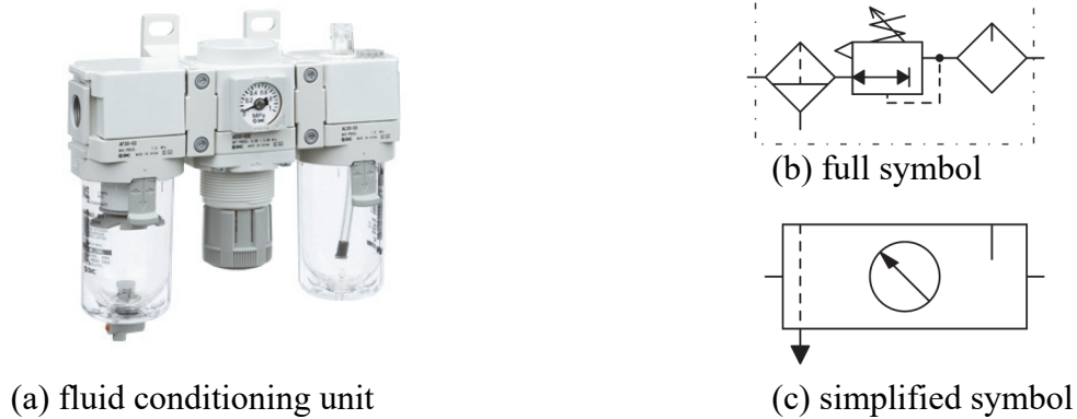
Figure 6.4. Fluid conditioning unit: (a) real [4], (b) full symbol, (c) simplified symbol
