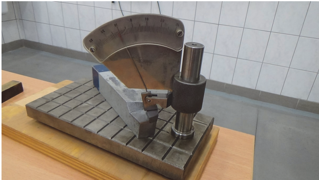
Figure 10.9. Special protractor for cutting tool angles measurements
