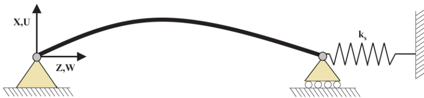
Fig. 1. The beam-spring system
