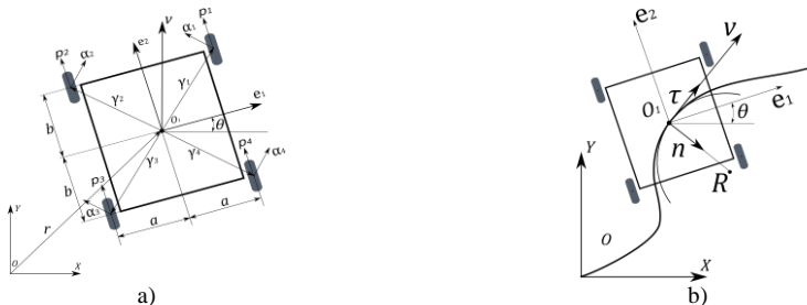
Fig. 1. a) The scheme of a mobile platform with omniwheels and b) curvilinear trajectory of motion
