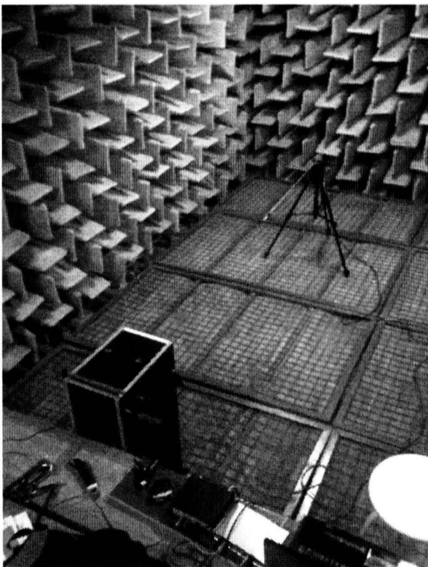
Figure 5. Measurement setup in an anechoic chamber.
