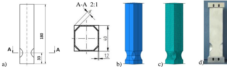
Fig. 1. Column models: a) general view, b) geometrical model in Abaqus FEM system, c) FE model, d) specimen A30 installed in blocs with vents
