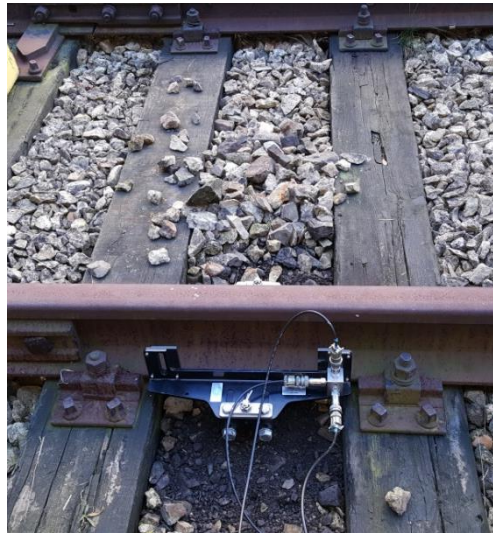
Fig.3. Specially mounting kit for accelerometers
