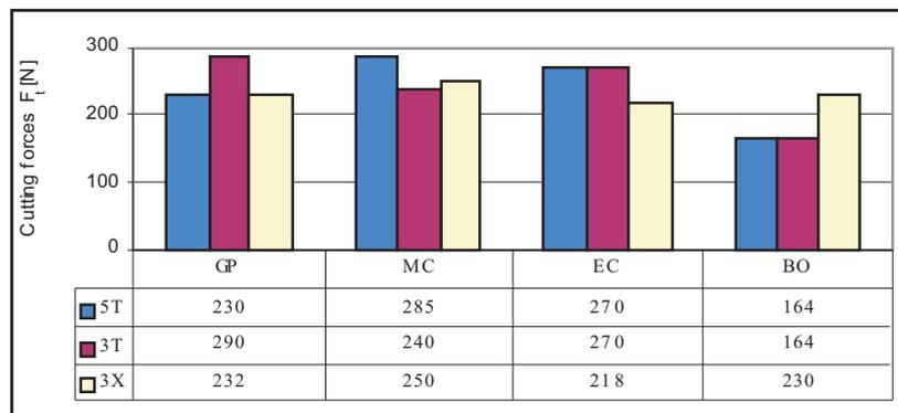
**Figure 2** The forces used by grinding wheels (5T, 3T, 3X) with the use of cutting fluid with MQL for alloy (P)
