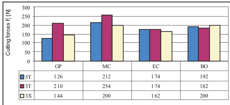
**Figure 1** The forces used by grinding wheels (5T, 3T, 3X) with the use of cutting fluid with MQL for alloy (T)
