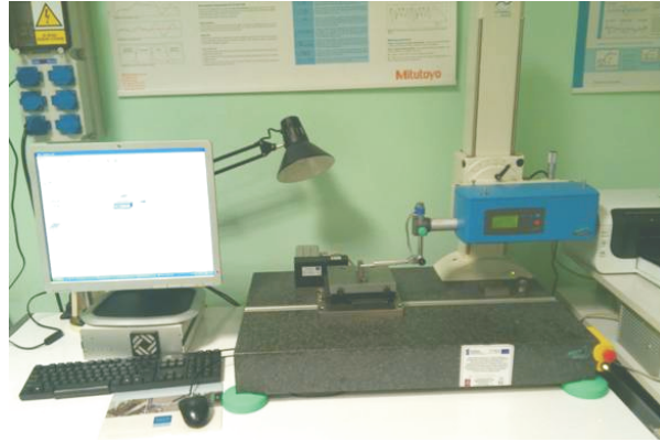
Figure 6 Measuring position- Profilograph TurboWaveline60
